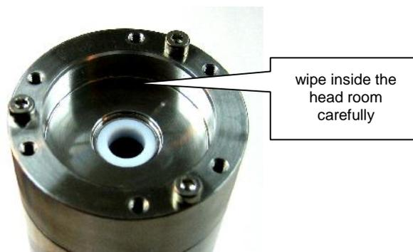
Put back in place first the support ring, then the sintered disc, and finally a new membrane. Place the membrane as flat as possible (smooth with finger is possible)
