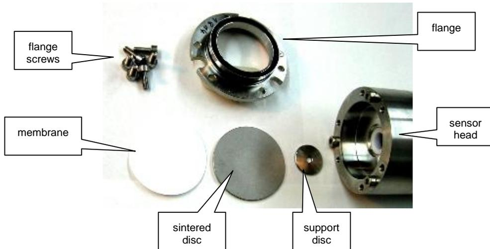
The flange has a side seal-ring and a membrane seal-ring.
