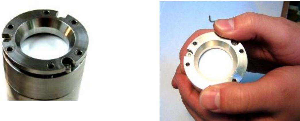
Align the flange to have the indentation covering the 3 head screws. Press the flange evenly gently down until it sits, avoid slanting.
