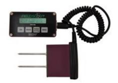
VWC varies depending on soil type. To overcome this variability, RWC normalises the data so wilting point is 0% RWC and a saturated soil is 100% RWC. Once the values of 0 and 100% RWC have been determined, the type of soil that is being measured is no longer of relevance.
