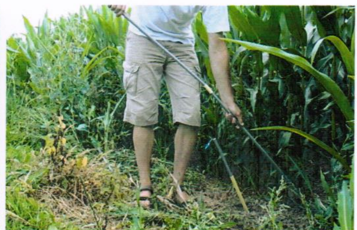
Extend this pipe with the other one and place it in the soil along the MacroRhizon. The lower end of the 2 meter pipe should be at the same level as the porous part
