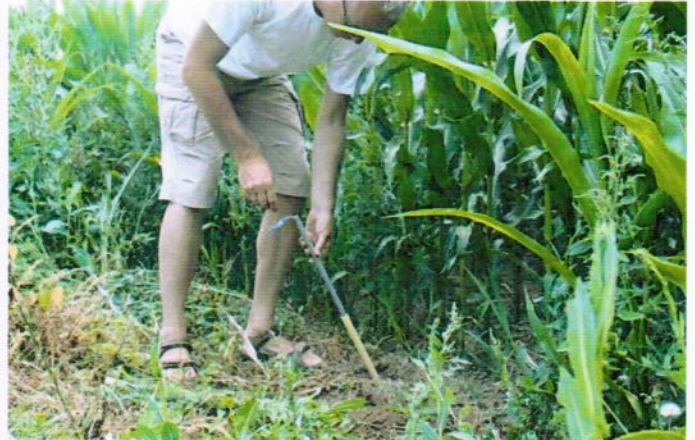
Put the MacroRhizon into the guide pipe and push the porous part carefully into the soil
