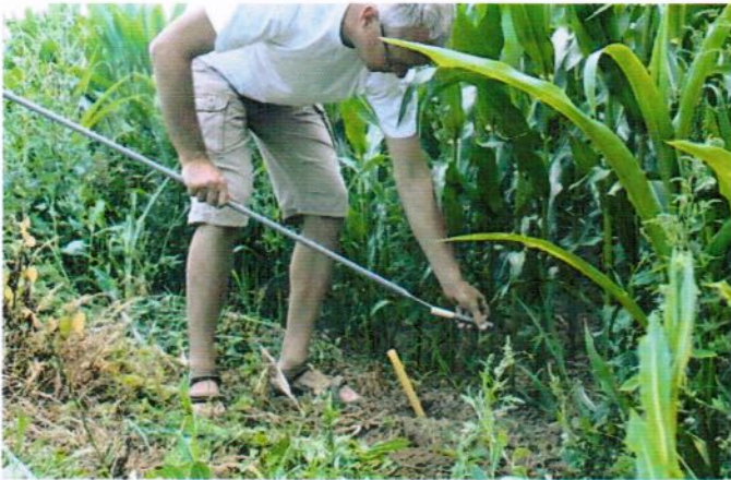
Remove the protection cap from the MacroRhizon
