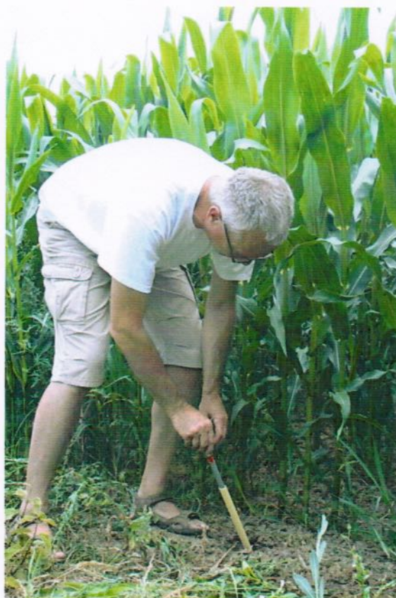
Put the insertion tool (pipe with steel pin) into the guide pipe and push the pin into the soil. Remove the insertion tool.
