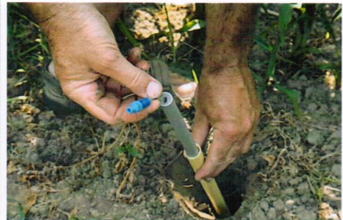
Remove the guide pipe and put the stopcock back
