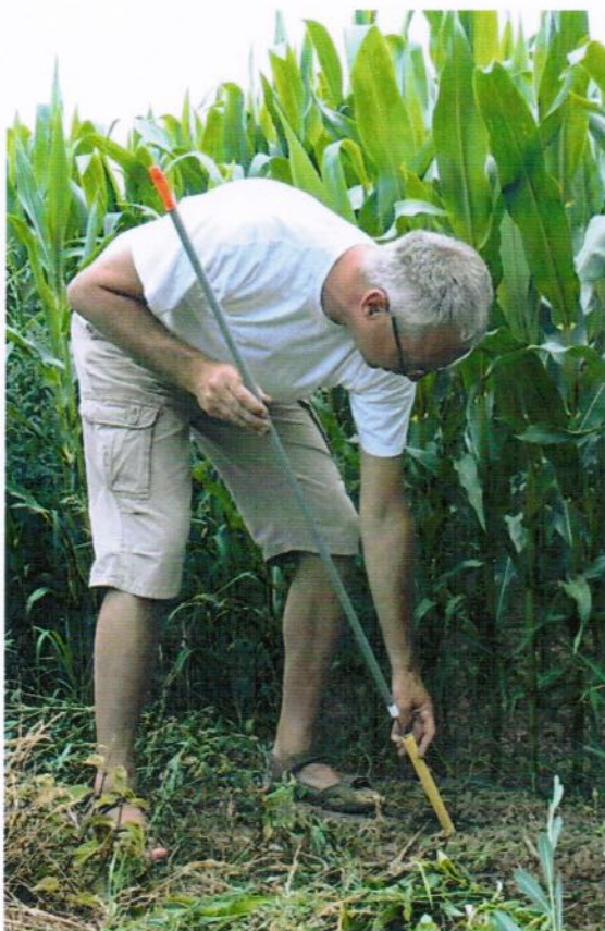
Put the insertion tool (pipe with steel pin) into the guide pipe and push the pin into the soil. Remove the insertion tool.
