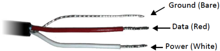
Figure 2: Pigtail End Wiring
