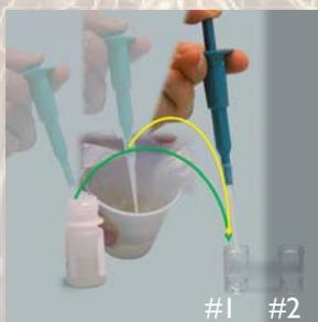
5. Add 800 µL Buffer to vial, then using a new pipette tip, add 200 µL sample; stir well with pipette tip
