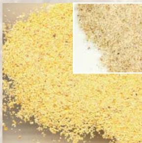
1. Collect and grind representative sample to a fineness of 20 mesh per Product Insert instructions
