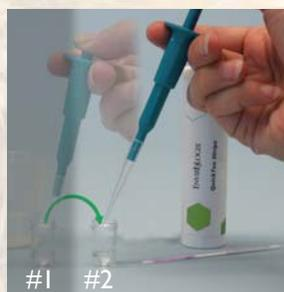
6. Transfer 200 µL of mixed sample to the second reaction vial used for testing
