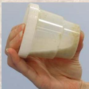
3. Shake on mechanical shaker (or vigorously by hand) for 30 seconds. (Oats & white wheat flour, shake for 1 minute.)
