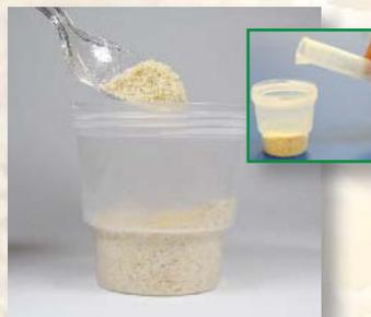
2. Add a 20-50 gram sub-sample to container, then depending on commodity, add 4, 5 or 6 mL/gram room temperature bottled/distilled/deionized water (eg: DDGS, 20 grams x 4 = 80 mL)
