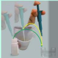
Add Buffer to Dilution Vial first, then add extract; mix well with pipette tip (Step 6,7)
