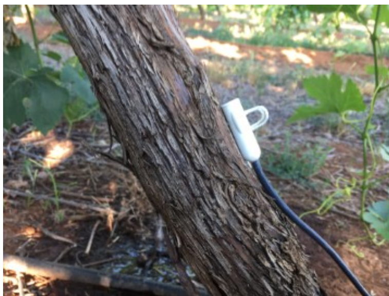
Figure 2. Needle misalignment can occur even when extreme care is taken with drilling and the installation process. Grapevines, such as seen here, can be difficult as well as installing a sensor where the trunk is at an unusual angle.
