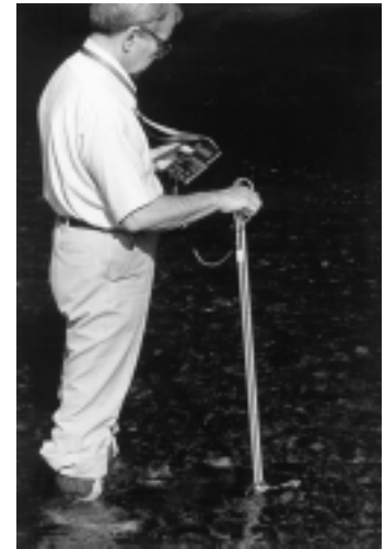
2100-12, quick profiling of shallow streams
