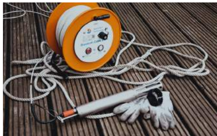
CTD48, Bluetooth Cable Drum and Sea & Sun DataWatch Photo: Sea & Sun Technology GmbH
