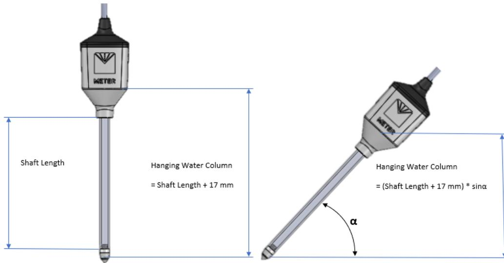
Figure 18 Position of reference point for water potential measurement
