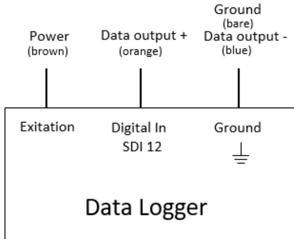
Figure 8 Wiring diagram SDI-12
