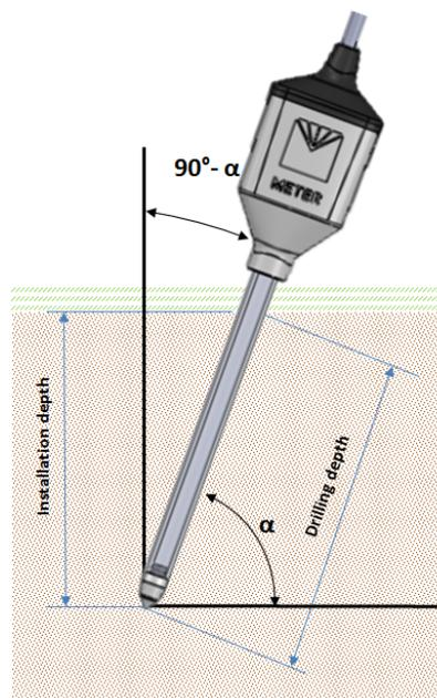
Figure 1 Drilling depth depending on installation angle
