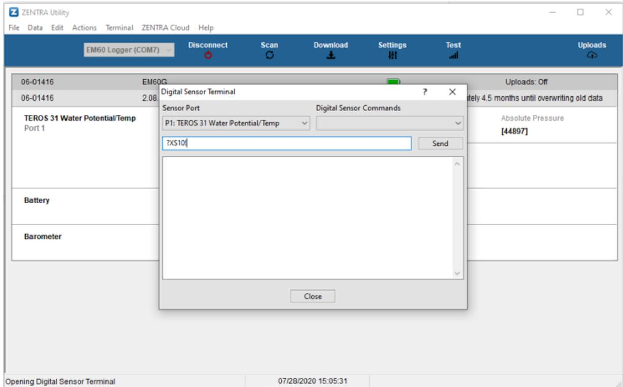
Figure 17 send shaft length command to TEROS 31
