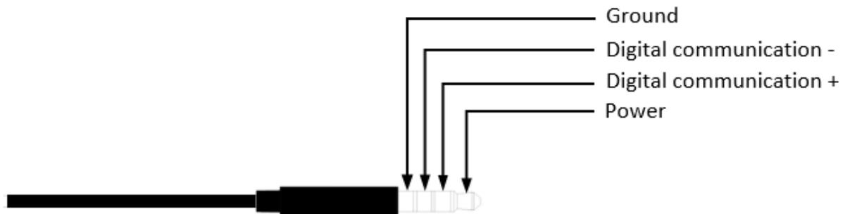
Figure 6 4-pin Stereo plug connector
