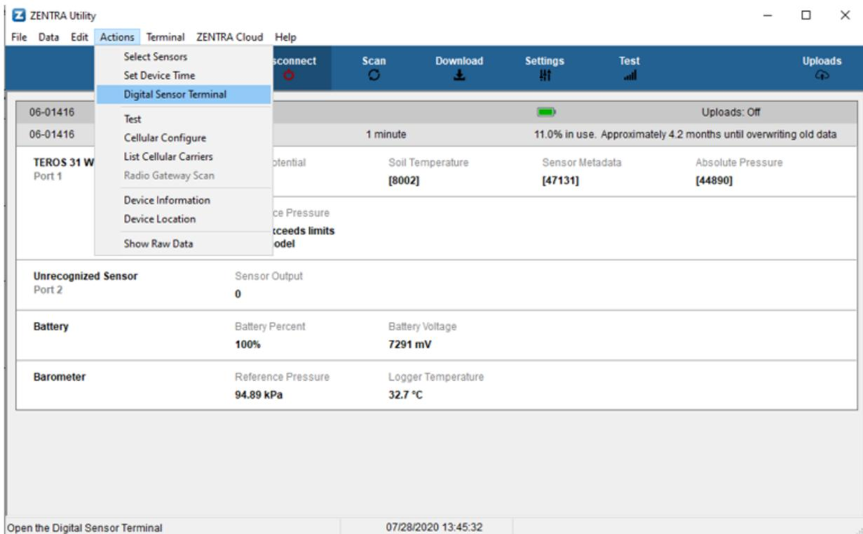
Figure 16 open Digital Sensor Terminal in Zentra Utility
