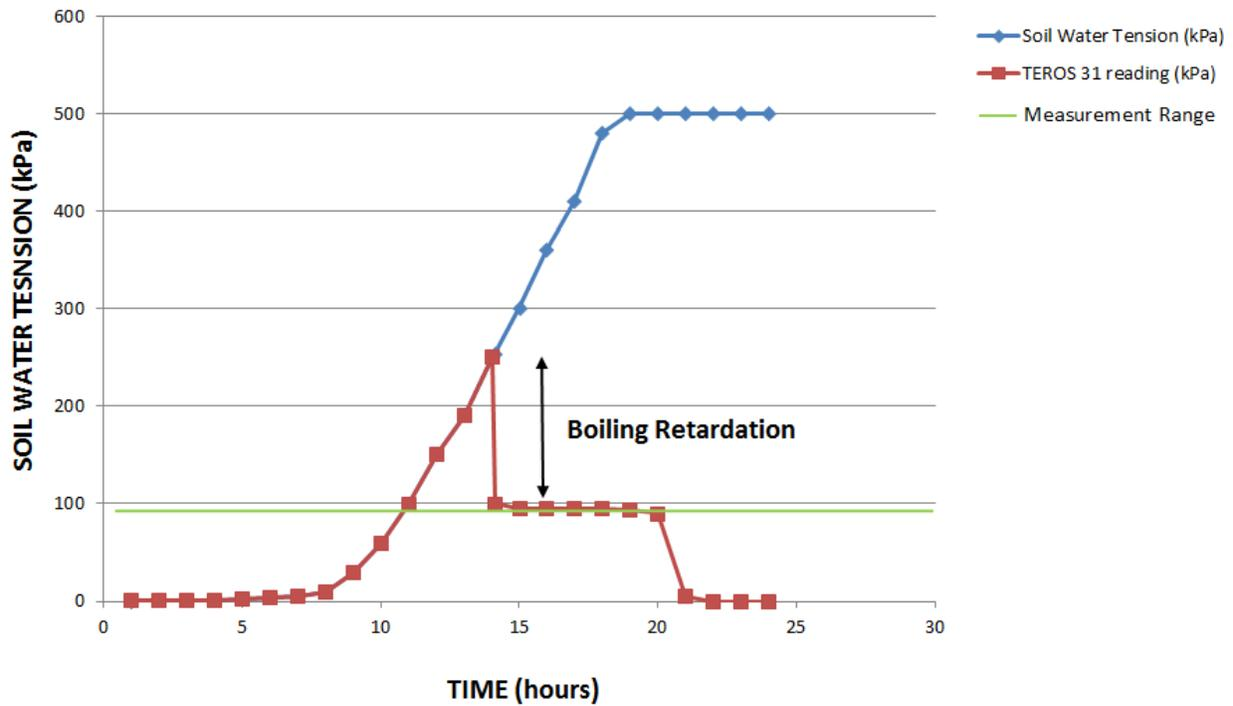
Figure 14 Tensiometer readings with boiling retardation
