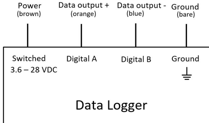
Figure 9 Wiring diagram RS-485
