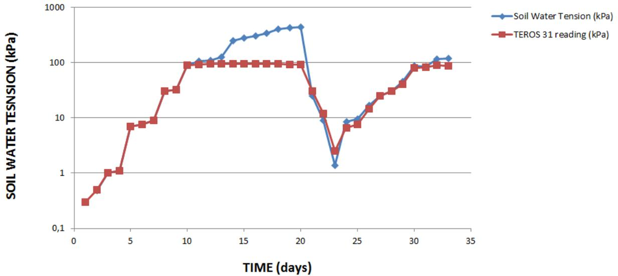
Figure 13 Tensiometer readings with tensions to -400 kPa
