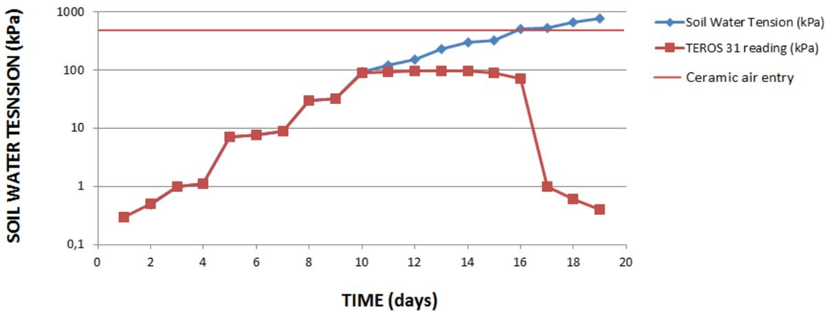
Figure 12 Tensiometer readings with tensions to -1000 kPa
