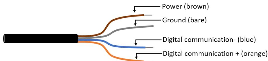
Figure 7 Pigtail wiring
