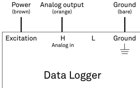
Figure 3 Wiring diagram
