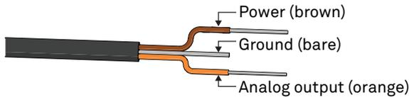
Figure 2 Pigtail wiring
