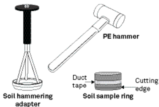
Figure 6 METER soil hammering adapter and hammer
