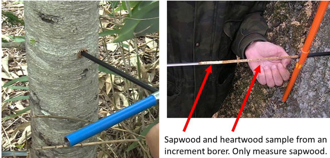
Figure 5. An increment borer is shown taking samples of sapwood within a tree.
