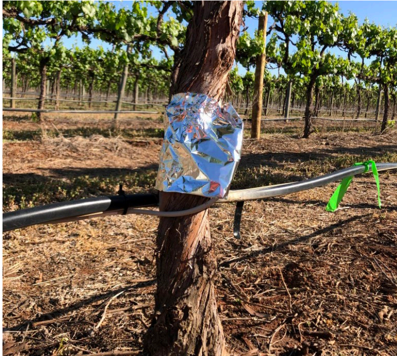
Figure 16. A sensor with insulation. DO NOT CABLE TIE THE SENSOR DIRECTLY AGAINST THE TREE!
