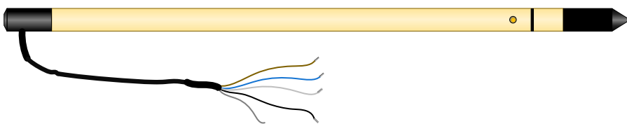
Figure 3. ORP-30-1-A (A type soil Redox probe).
