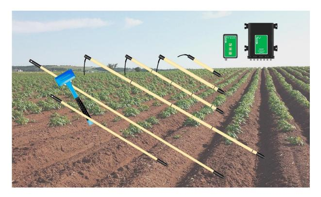
With our innovative soil Redox probes, soil oxidation and reduction potentials can be measured accurately in laboratory, agricultural, environmental and industrial applications. The SWAP soil Redox probes contain single or multiple Pt electrodes in different configurations, with or without integrated reference electrode and temperature sensor. Accuracy, durability, versatility, low maintenance at a cost-effective pricing! It is connectable to a wide range of data loggers.
